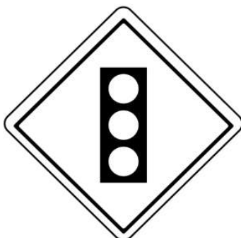
TRAFFIC SIGNAL AHEAD Figure 15-8
